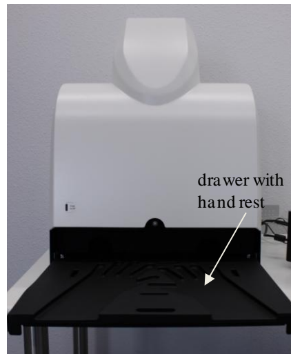
Figure 2-4 View of the Xiralite® Fluorescence Imager X4 with opened flap and pulled out drawer with hand rest.
